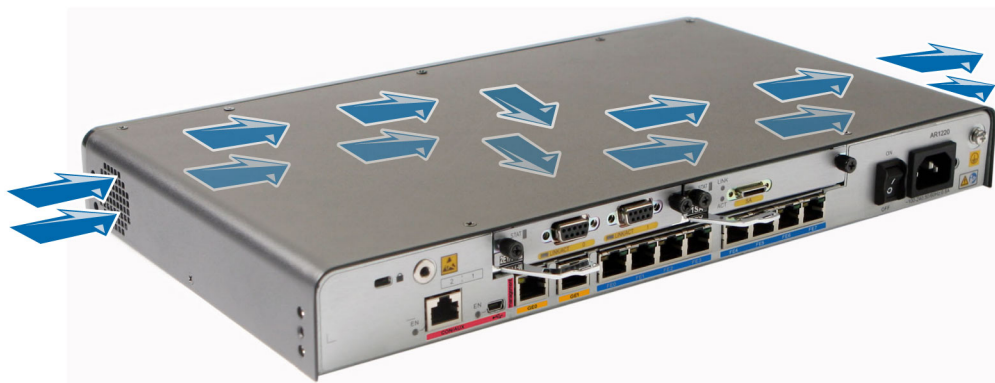
Figure 4-1 Air circulation through the AR1200 chassis
