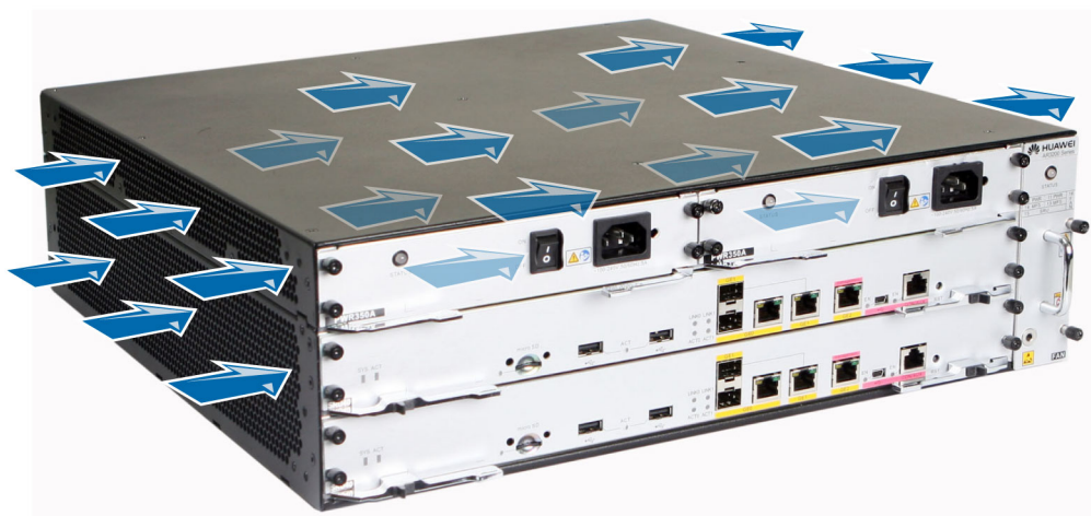
Figure 4-4 Air circulation through the AR3260 chassis
