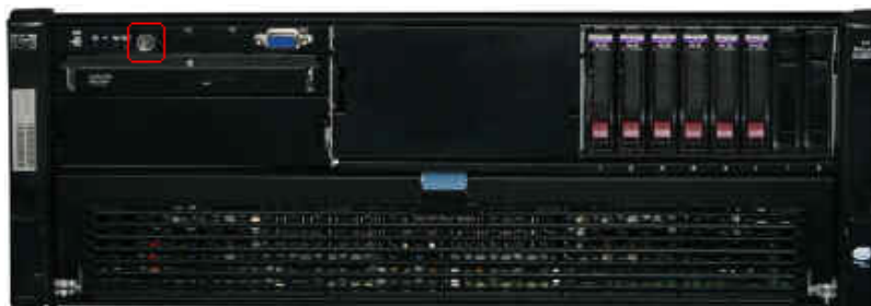
Figure 4-1 Position of the power button of the DL580G5 server
