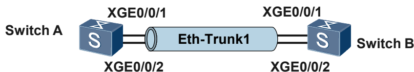
Figure 3-5 Network diagram of Eth-Trunk load balancing
