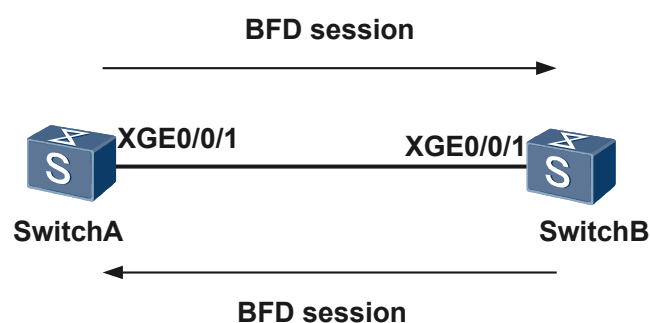
Figure 6-10 Networking diagram of BFD for PIS
