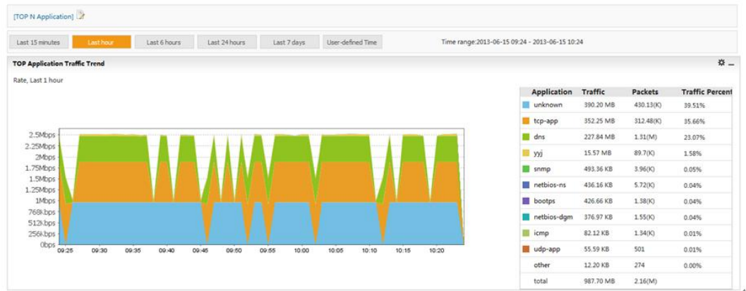
Figure 4-138 Application traffic analysis
