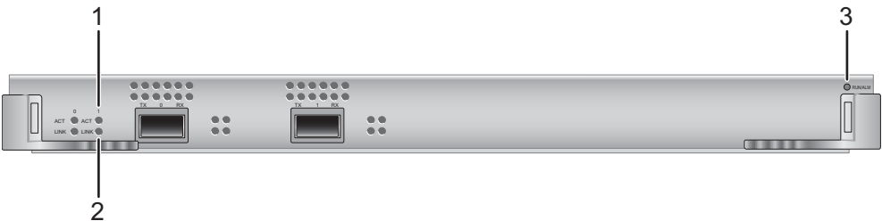
Figure 6-124 Indicators on the ES1D2L02QFC0 panel
