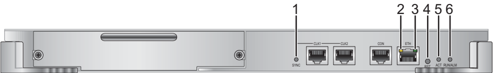
Figure 6-6 Indicators on the ES0D00SRUB00 panel
