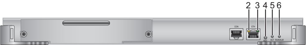
Figure 6-5 Indicators on the ES0D00SRUA00 panel
