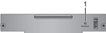
Figure 6-15 Indicator on the ES0D00FSUA00 panel
