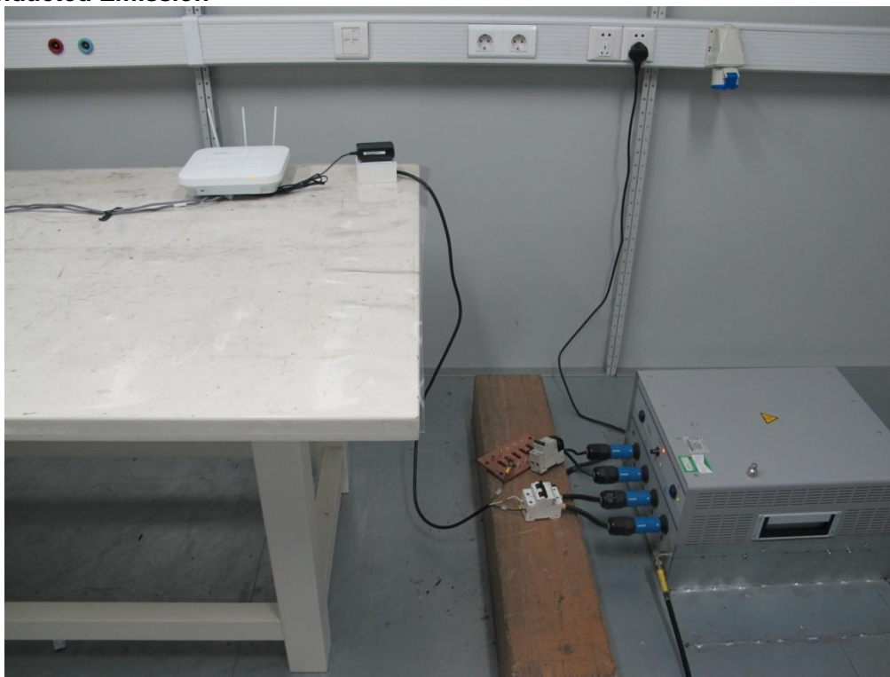
Conducted emissions of AC power port
