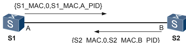
Figure 8-8 Exchange of initialization messages
