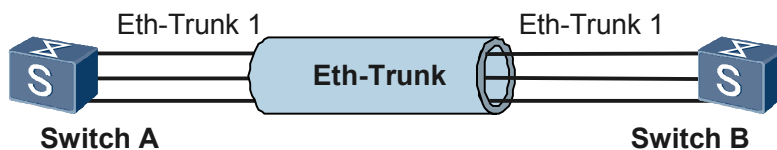
Figure 3-6 Link aggregation in manual load balancing mode network diagram
