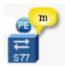
Figure 10-120 Highest L3VPN alarm severity on a PE
